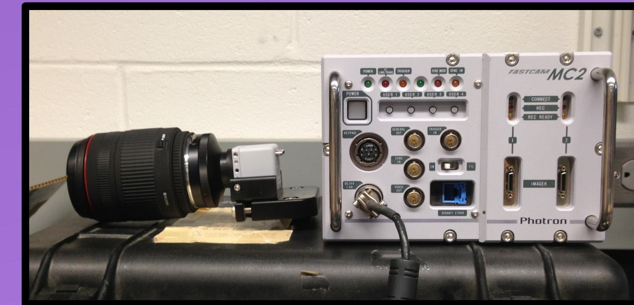
Figure 5: Photron Fastcam MC2 high-speed camera set up uses a modular computer system which internally saves 4,000 frames. The camera is capable of 2,000 fps, though in low-light setting can only do up to 20 fps, making it impractical for our quick flash.
