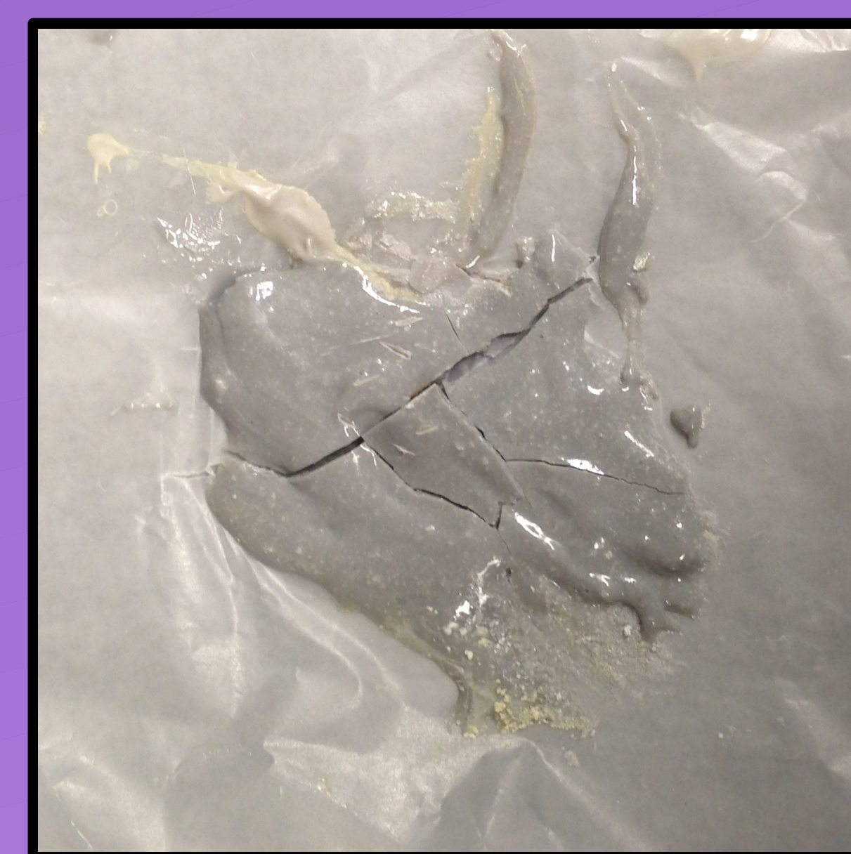
Figure 6: Specimen of BAS powder mixed with metal epoxy. Crack was induced in a dark room, but no discernible emission of light could be detected.
