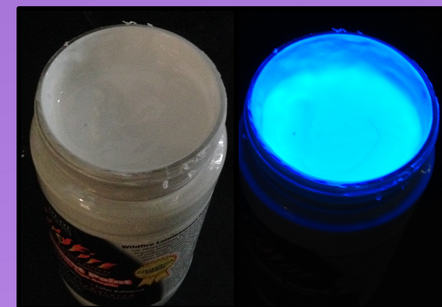
Figure 7: WildFire UV paint at rest in dim room (left) and glowing under an ultraviolet light source (right). This is the same effect that makes things glow under a black light.
