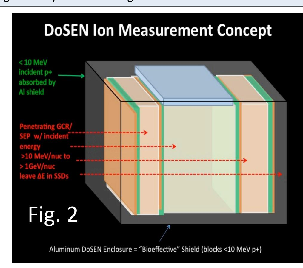
Ion Measurement Principle: For heavy ions and protons, DoSEN provides a direct measurement of the LET spectra behind shielding material (Fig. 2). For LET measurements, DoSEN contains stacks of thin-thick Si solid-state detectors (SSDs) similar in design to those used for CRaTER (Fig. 1). The thicknesses are 150  $\mu$ m (thin) and 1000  $\mu$ m (thick).
