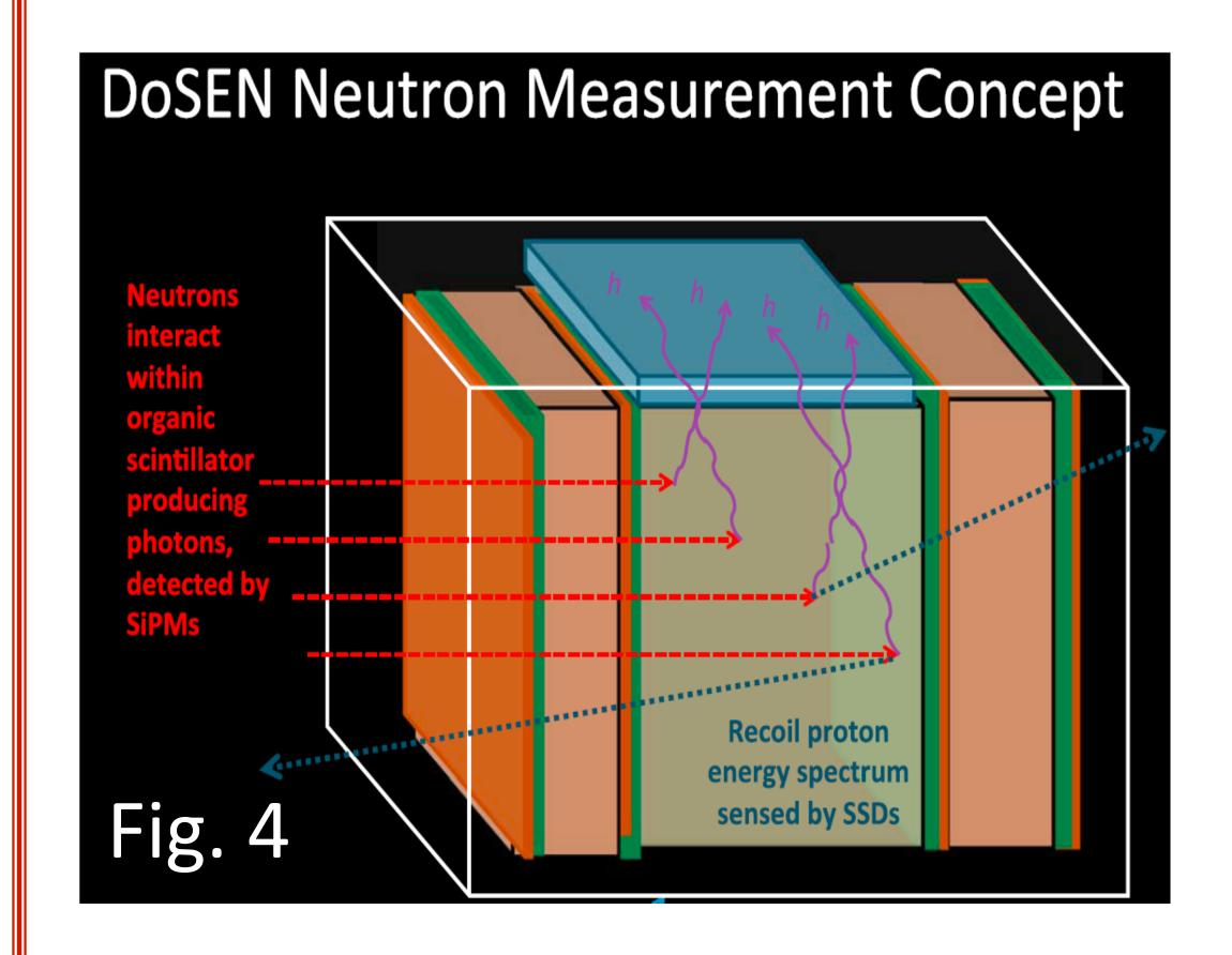
**Neutron Measurement Principle:** DoSEN also measures neutrons from 10 to 100 MeV, which requires enough sensitive mass to fully absorb recoil particles that the neutrons produce (Fig. 4). Organic stilbene scintillator is used to record neutron interactions, which can be distinguished from gamma-ray interactions via pulse shape discrimination (PSD). The scintillator light is recorded using com- pact, low-voltage silicon photomultipliers (SiPMs) [*Bloser et al. 2013*]
