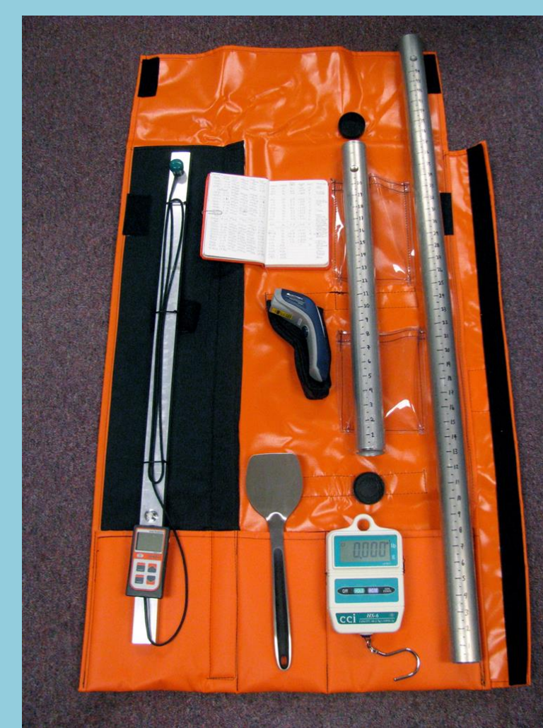
Figures 4 & 5: Measurements are taken of: 1. Albedo 2. Snow depth 3. Snow weight 4. Surface Temperature 5. Cloud cover/weather observations
