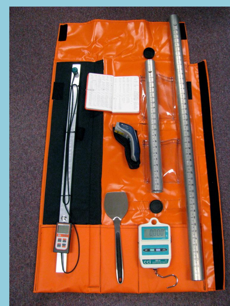
Figure 3 (right): "Albedo kit" includes temperature gun, pyranometer, snow tubes, hanging scale, log book and spatula.
