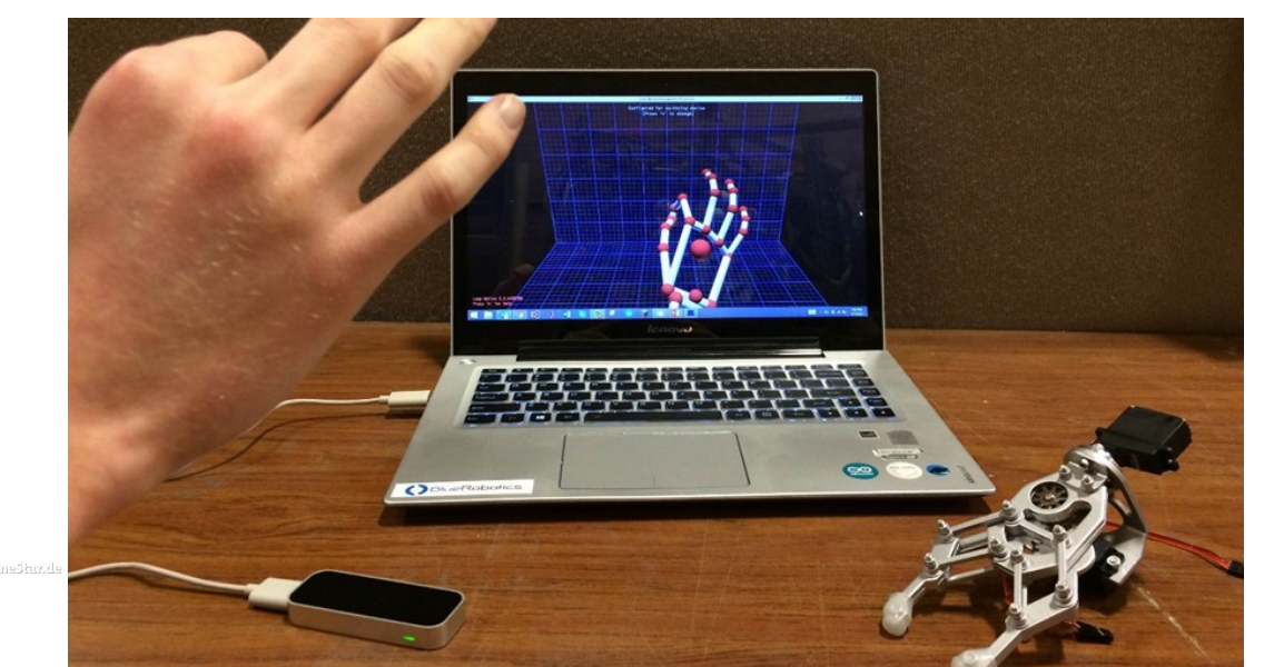
Leap motion & Xbox 360 controllers provide the bulk of the human interaction with the ROV
