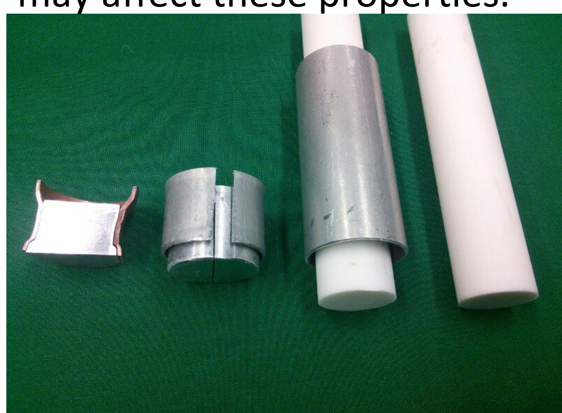
Impacted metal samples on the left, unimpacted ceramic samples on the right.
