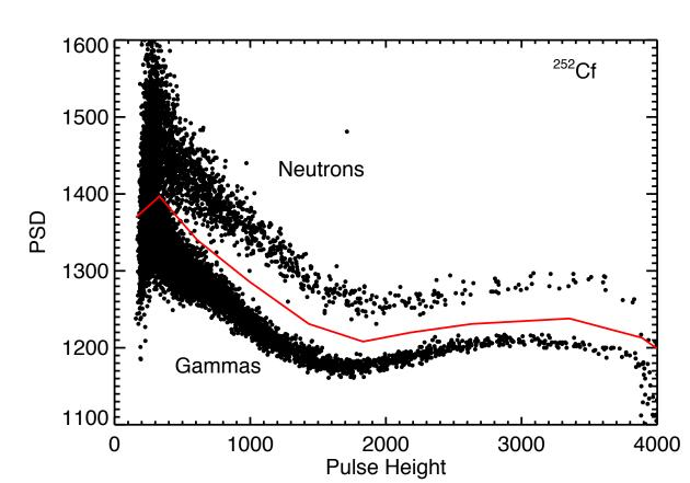
P-terphenyl PSD response determined with <sup>252</sup>Cf fission source.
