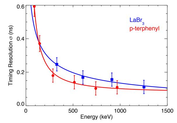
ToF contribution from individual scintillator elements based on calibrations using coincident gamma rays from <sup>60</sup>Co source.
