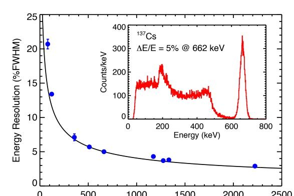
LaBr<sub>3</sub> calibrated up to 2.2 MeV with gamma ray calibration sources.
