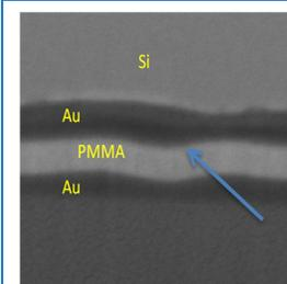
We next investigated deposition of the PMMA by pulsed laser deposition (PLD), which is carried out in a vacuum chamber and compatible with the MS deposition method. Polymer/metal multilayers can be grown by PLD with high quality only if the polymer film has sufficient hardness to resist the stress in the metal layers. Our PLD-deposited PMMA films were too soft to obtain a good multilayer.
