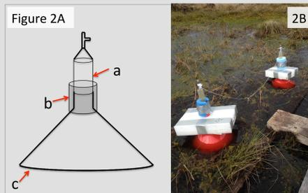
Figure 2. A. Diagram of manual bubble traps deployed in each pond (a: 60mL syringe with stop-cock; b: flexible tubing; c: 25cm plastic funnel). 18 bubble traps deployed in 6 ponds each summer since 2012. B. Two bubble traps deployed in a Stage 1 pond.
