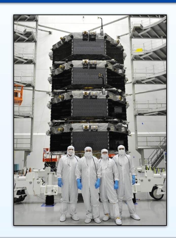
MMS was launched in 2015 to study magnetic phenomena in the Earth's magnetosphere. Four identical spacecraft carry a total of 28 flight instruments that were designed and fabricated at UNH.
