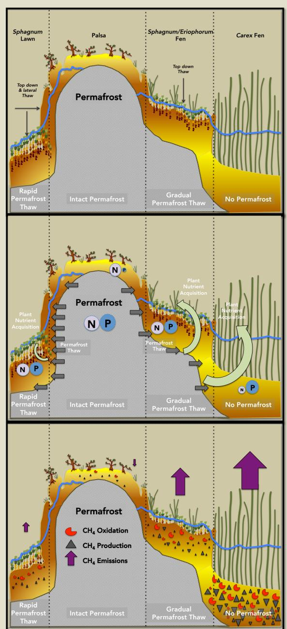
Figure 2. Conceptual diagram of wetland types and nutrient and methane dynamics impacted by permafrost thaw
