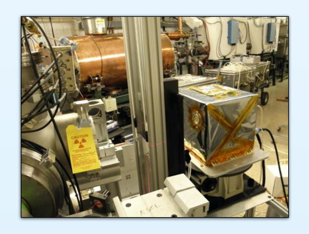
The energetic heavy ion sensor (EHIS) space weather instrument was designed, built and calibrated at UNH for the GOES-R weather satellite, which was launched in November of 2016.
