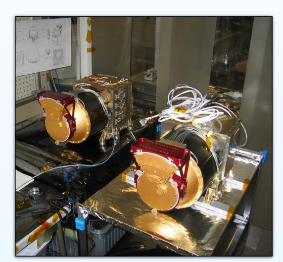
Launched in 2006, the two spacecraft STEREO mission a stereoscopic (3-D) view of the Sun and the interplanetary space environment. UNH provided, for each spacecraft, the The Plasma and Suprathermal Ion Composition (PLASTIC) instrument samples the solar wind and energetic particles.
