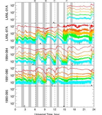
Figure 1. LANL geosynchronous data showing four sawtooth injections during the event. Injection time is marked by dashed blue lines. FAST passes are shaded by gray bars
