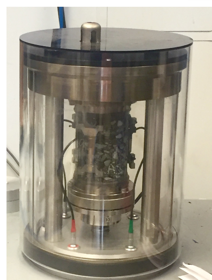
Asphalt sample with LVDTs
