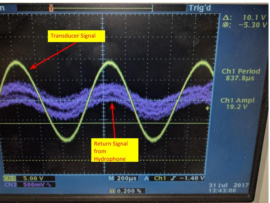
• Transponders are judged by their Transmitting Voltage Response (TVR). • Calculated by TVR = SL -  $20\log_{10}V_{drive}$
