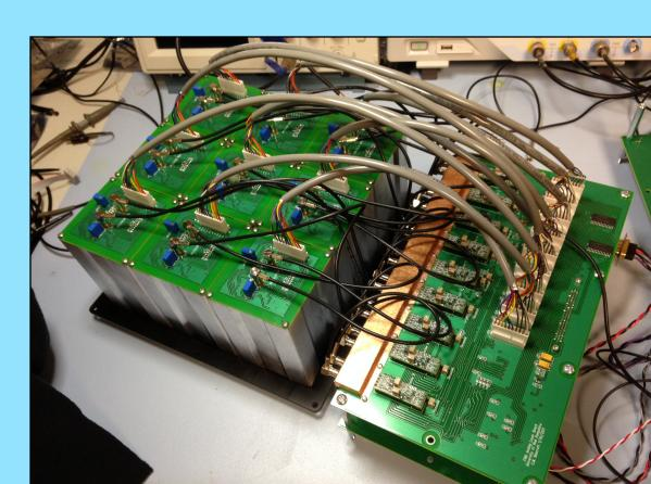
Layer arrays contain nine detector cells with discrete readout
