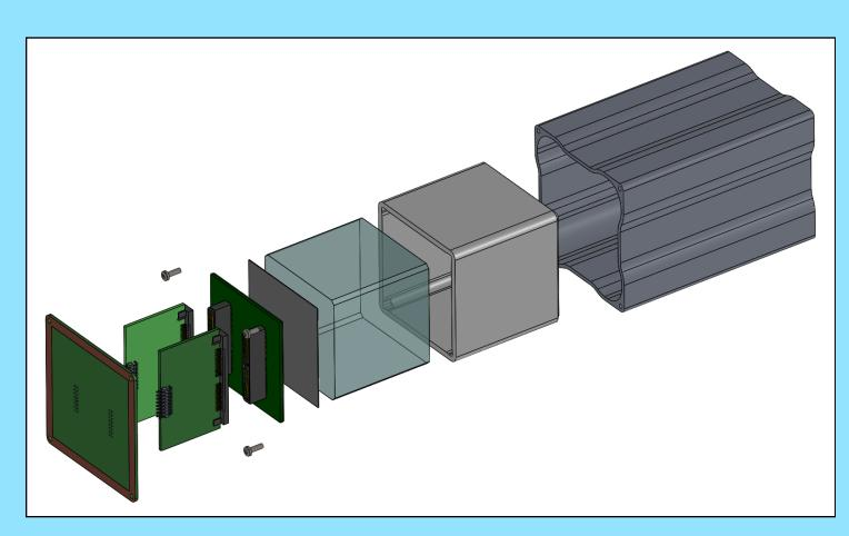
Detector cells constructed with plastic scintillator and SiPM arrays
