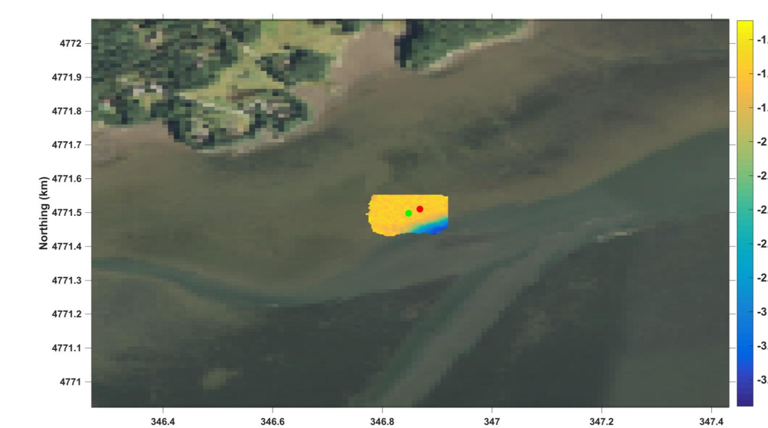
Figure 4: Multibeam survey bathymetry collected at area surrounding Station B plotted on top of GIS image of the Great Bay. Red and green dots represent frame location, as the frame was deployed in a slightly different location in 2017 as in 2016.
