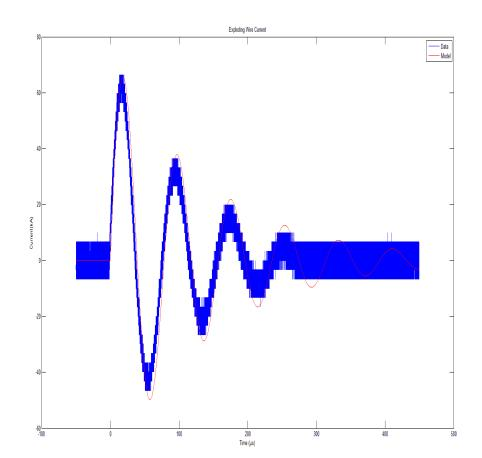
Current properties: f=1.27 kHzRise time = 19.6 µs  $\beta = 7000 \text{ rad/s}$ Rt = 6.03 m $\Omega$ Lt=430 nH  $I_{\text{max}_{\text{model}}} = 65.6 \text{ kA}$  $I_{\text{max}_{\text{data}}} = 66.4 \text{ kA}$
