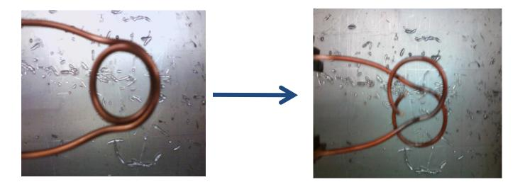
2.5 turn coil critical failure. Notice the remains are nearly equal in length. This demonstrates magnetic field strength is strongest at the center of the coil.
