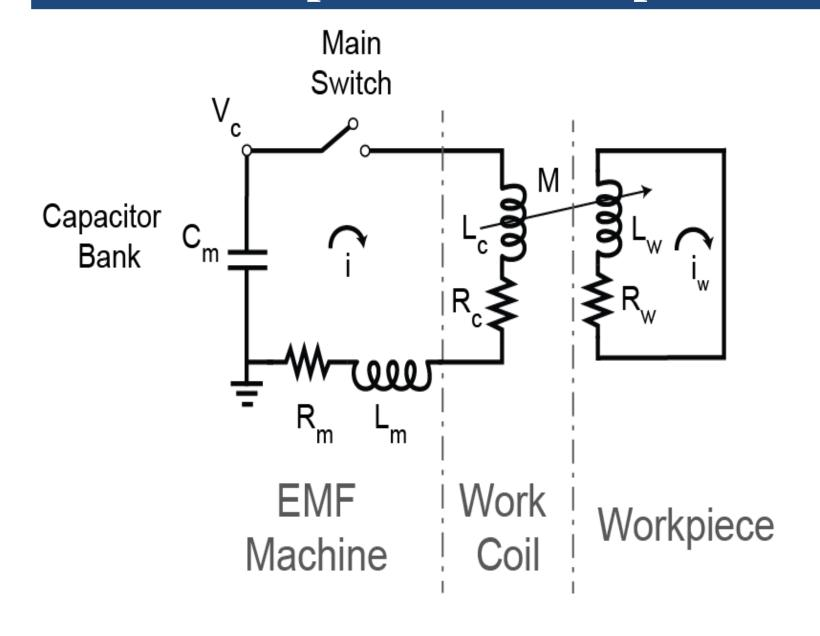
Experimental setup consists of a 12 kJ pulse generator. Once energy is charged in the capacitors  $C_m$ , current pulse runs through coil. In the presence of a workpiece a current is induced, contributing to the circuit through its mutual inductance with the work coil.
