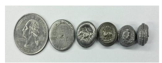
Example of EMF process from "shrunken quarter" experiments. As you can see the during the process the coil explodes violently. The coil is connected to the leads which are connected to our pulse generator (not shown).
