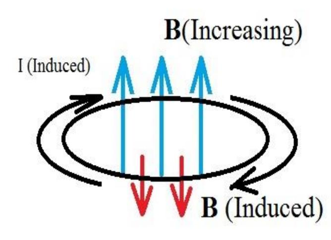
A conducting loop experiences an increase in magnetic flux through its surface. Lenz's Law states that the a current is induced in the loop as to oppose the change in magnetic flux.
