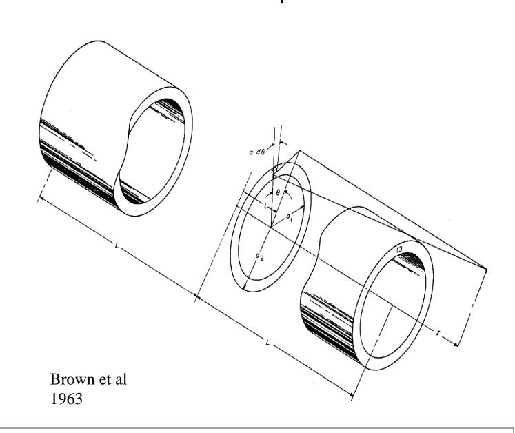
Coil geometry from [2]. Note they treat their coil as a long, solid conducting tube, however since our coils are tightly wound this is a sufficient approximation.
