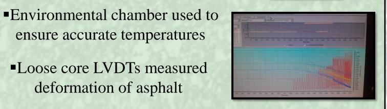
■Tested 5 specimen at 21 frequencies (Hz) and 5 temperatures (°C):
