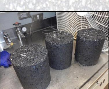
Asphalt Temperature 335°F discharge, 315°F compaction
