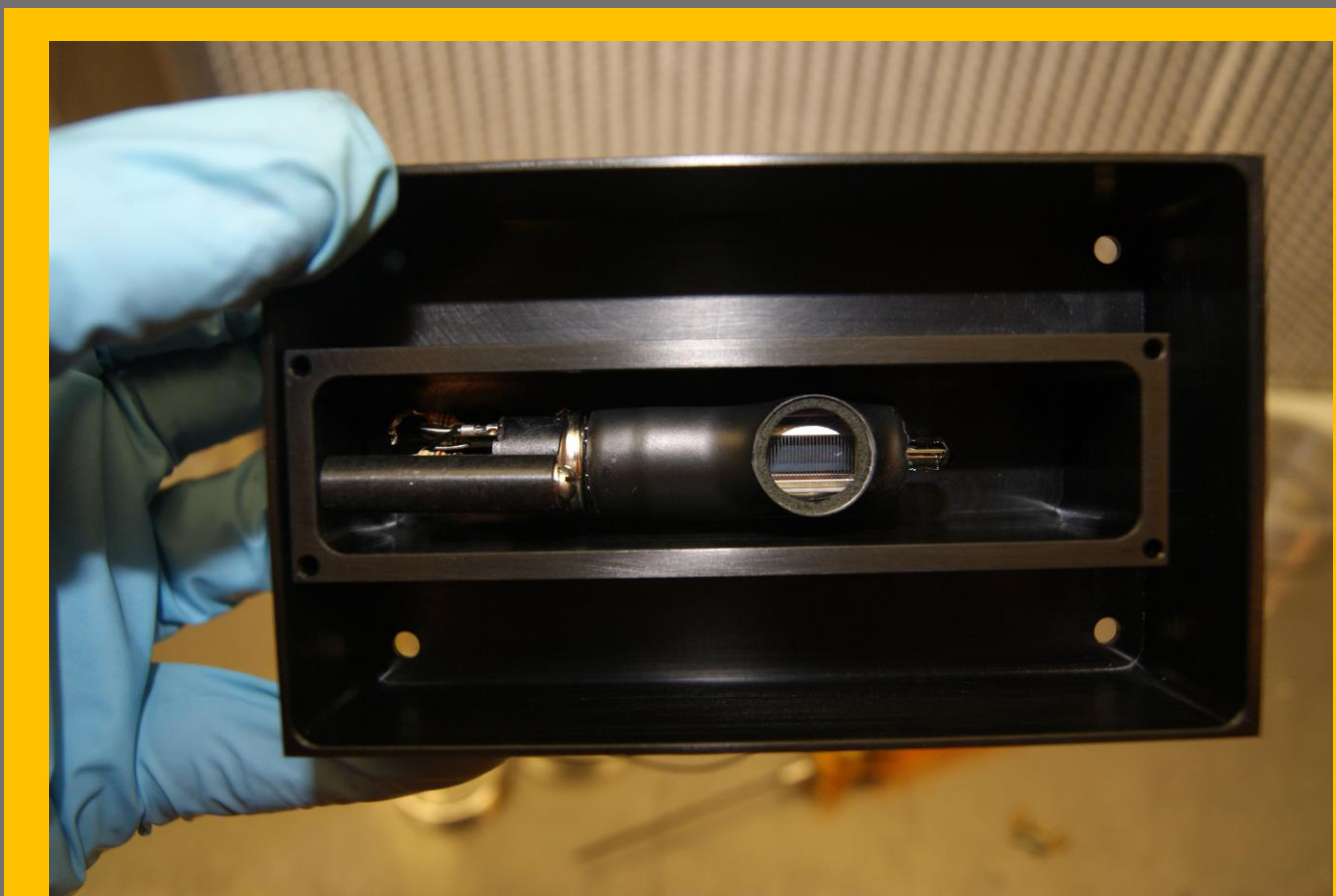
Fig 11. UV PMT with front baffle removed.
