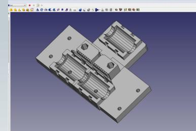
Figure 10: 3D printed Dual Mount
