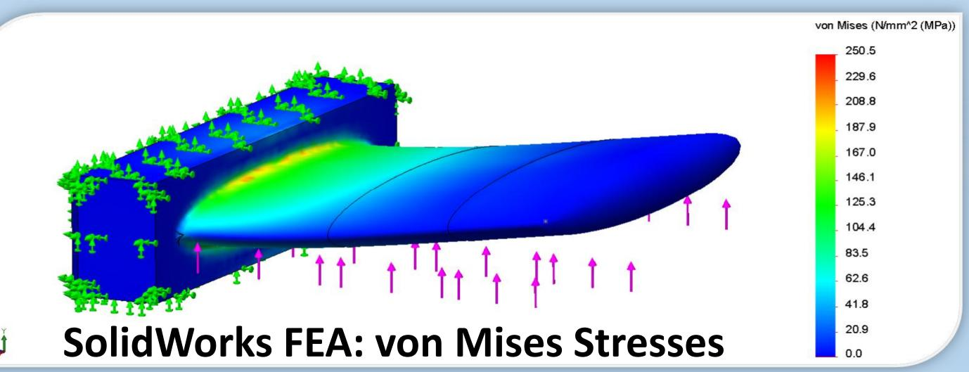
Stress and deflection analysis on experimental testing apparatus
