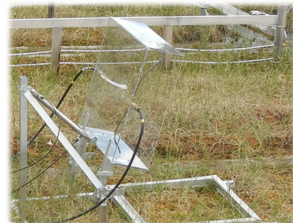
Fig. 4 Picture of an automated chamber located in the Sphagnum site
