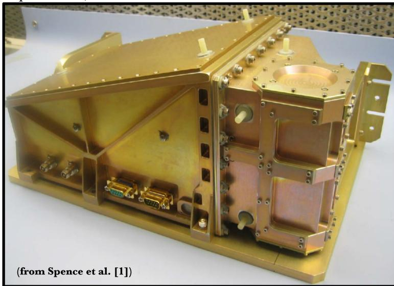
**Goals:** MPIRE investigates galactic cosmic rays (GCR), solar energetic protons (SEP), and secondary radiation produced at Phobos' surface using tissue equivalent plastic (TEP) to simulate astronaut self-shielding or shielding of a moderately thick spacecraft. MPIRE measures linear energy transfer (LET) spectra over a wide dynamic range behind different volumes of TEP and under different levels of solar activity and GCR flux.
