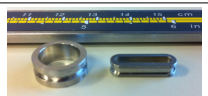
Figure 2: the two incoed cores used in the design of the sensor for the SIGMA mission
