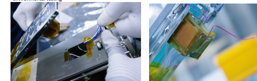
Figure 10: The Mini-fluxgate magnetometer being integrated onto the SIGMA CubeSat in South Korea for environmental testing
