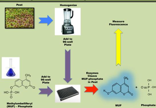
Figure 7. Enzyme assay schematic. Methylumbelliferyl (MUF) synthetic substrates fluoresce when enzymes cleave substrates in peat samples. Potential enzyme activity is then calculated based on fluorescent detection units and sample dry weights.
