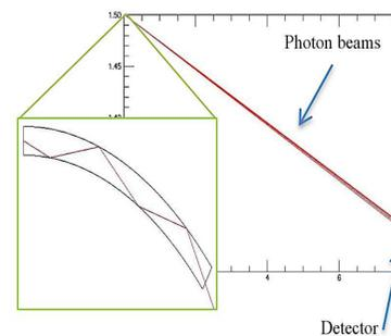
The channeling probability at 122 keV for a total bending angle of 0.4°, calculated for 200 nm layers of PMMA, Be, and C, shows that, while polymer would be optimal, C and Be perform nearly as well:
