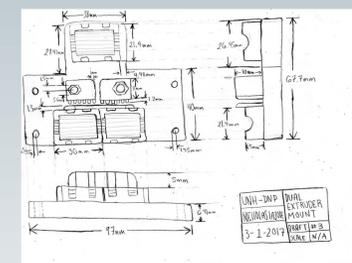
Figure 8: Drawing of Dual Mount
