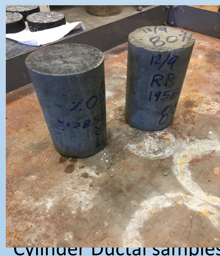
Cylinder Ductal samples
