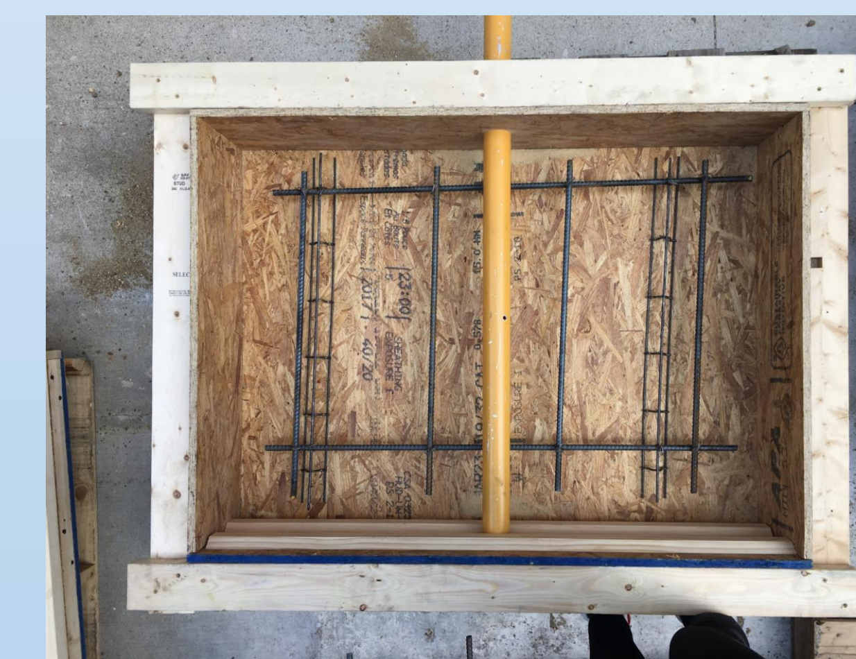
Test 3: T & G Post Tension Section
