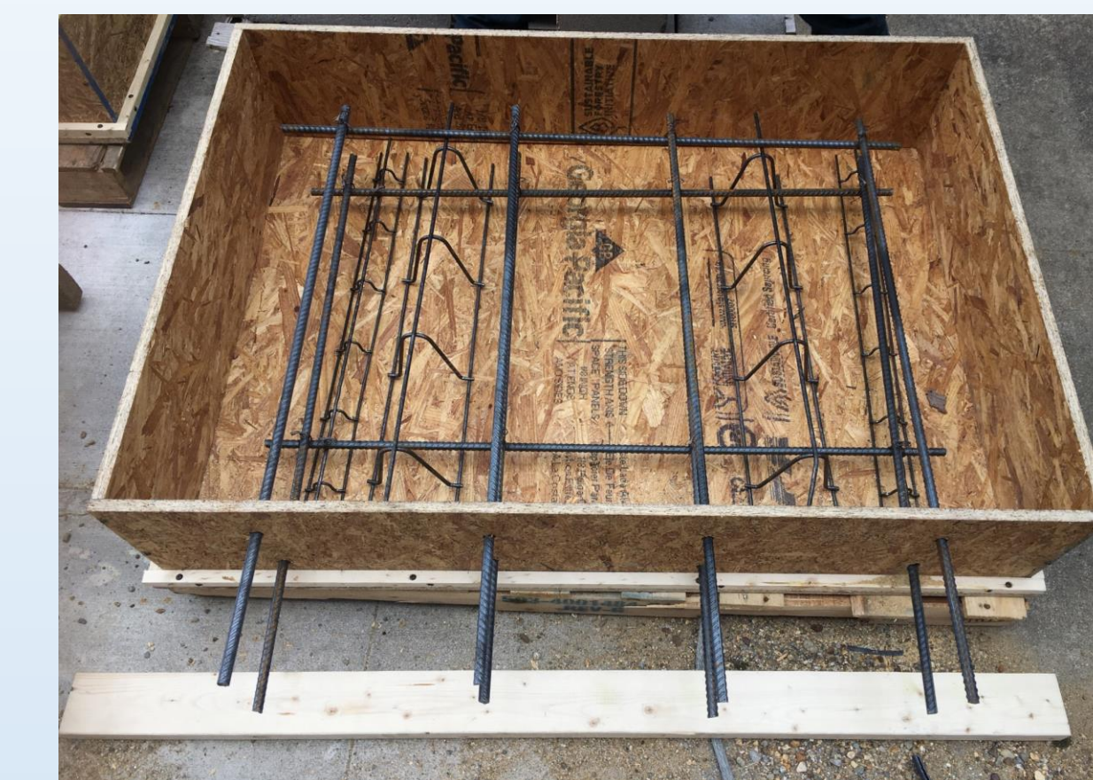
Test 1: Reinforced Joint Model Section
