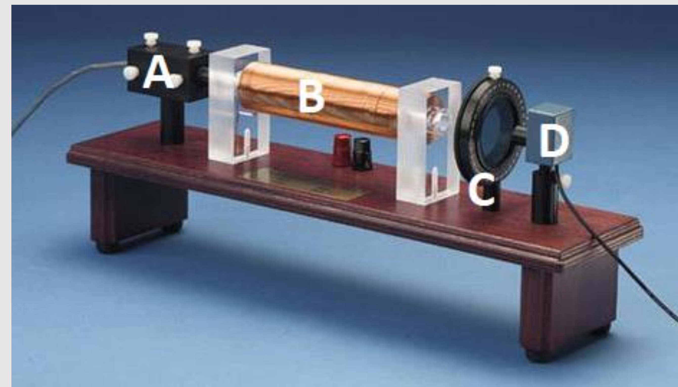
Faraday Rotation Setup used to measure the Verdet Constant
