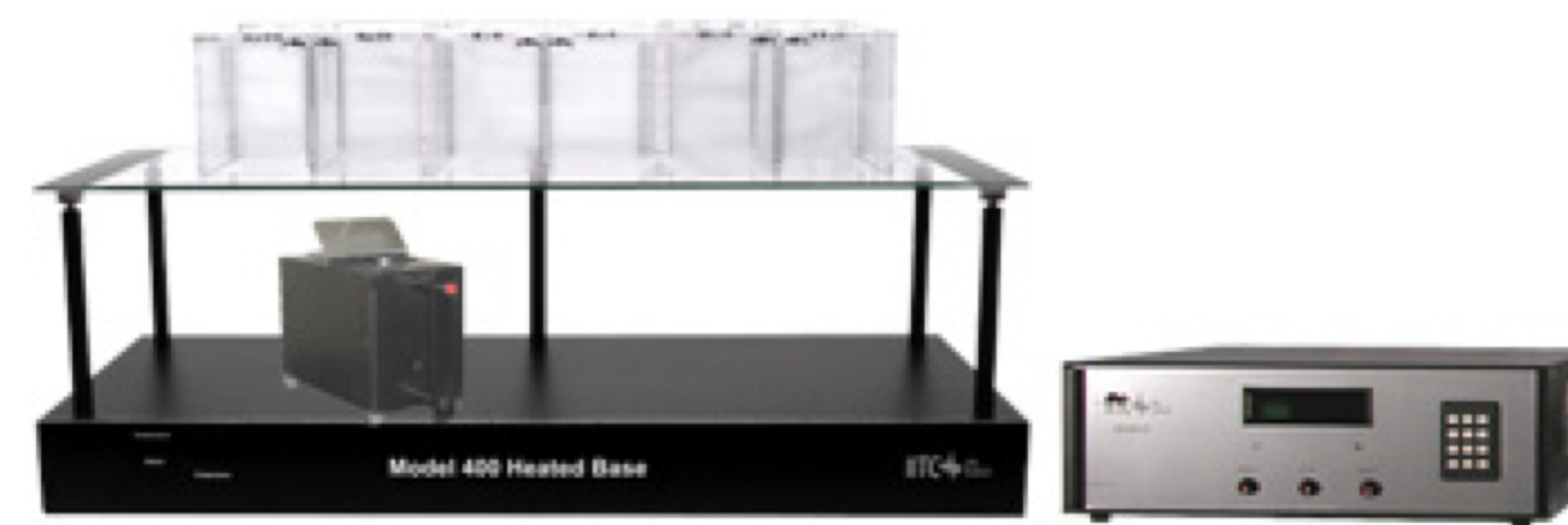
Figure 4: Shows the set up for the Hargreaves testing apparatus. One mouse is placed in each testing chamber, allowing up to twelve mice to be tested at once.
