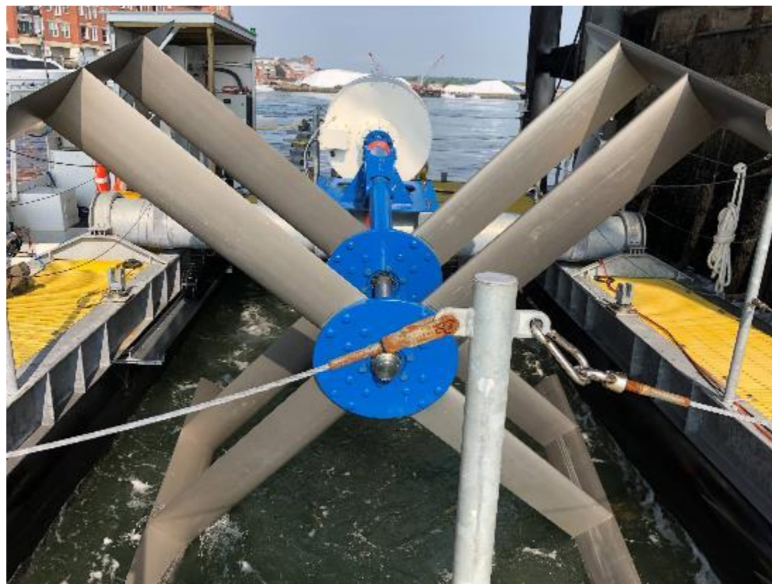
Figure 2: The Living Bridge Turbine
