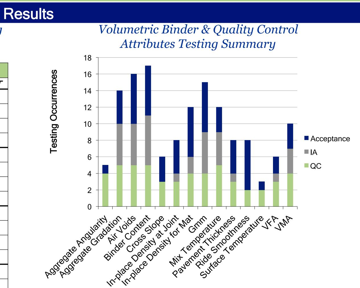
Observations from Attributes Testing Itemization & Summary: • Some attributes (*Binder Content, Air Voids, Gmm, Aggregate Gradation*) are tested at every stage of the QA process and/or by most states. This consensus makes them not an area of focus.
