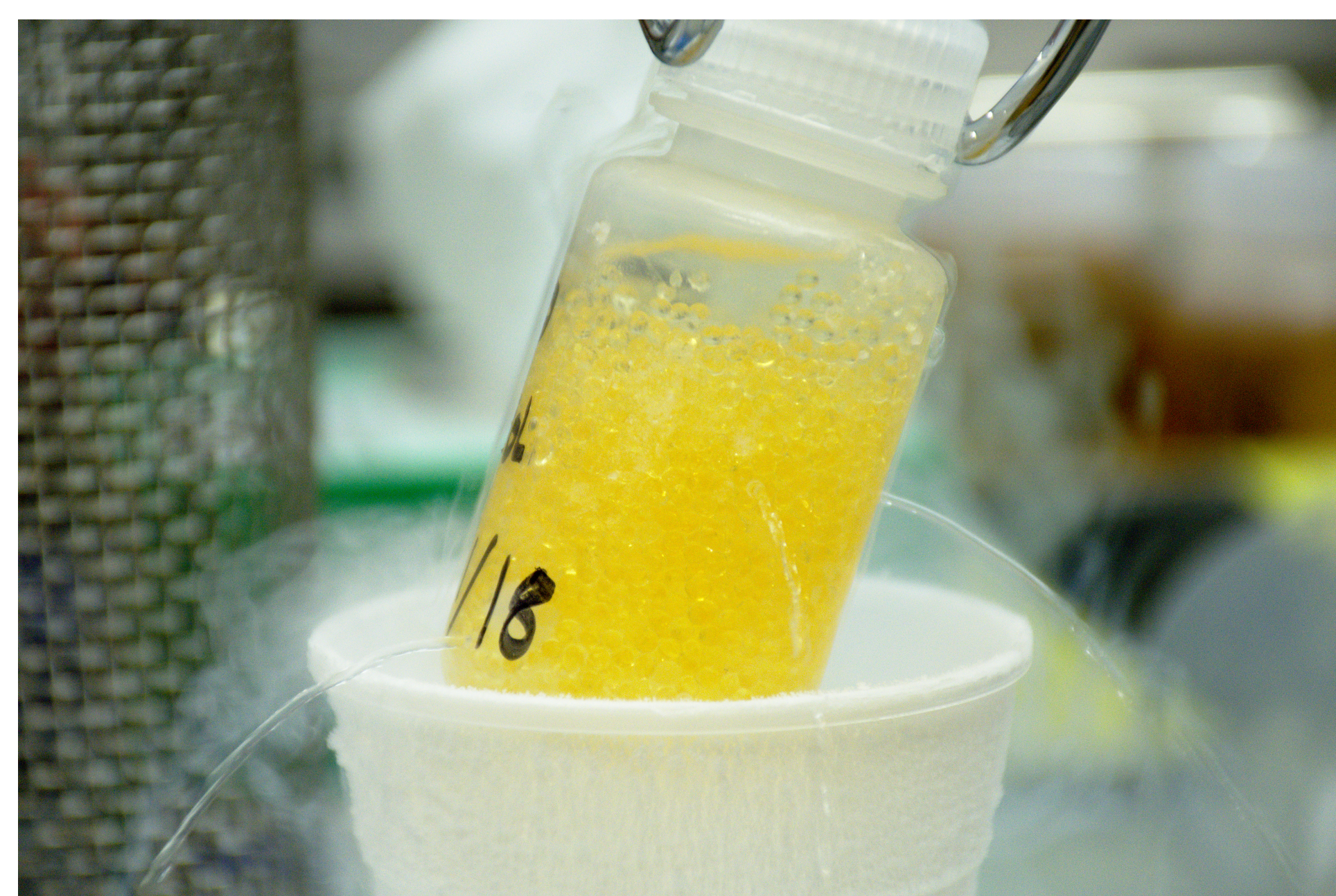
Figure 4: Frozen TEMPO doped n-butanol in storage vial. Prepared for long-term storage. This is the sample of n-butanol that the polarization data was measured from. See figure 5 for this sample's polarization measurements.
