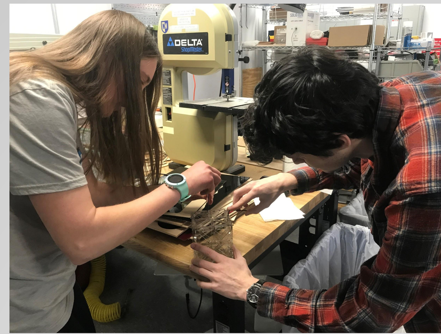
Pictured above: Chris and Eleonora countersink and assemble a laser cut acrylic model at the UNH Makerspace. The acrylic model is the easiest to manufacture with on-campus facilities and minimal training.
