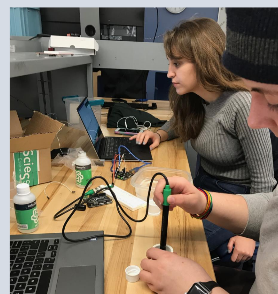
Calibrating the sensor with known concentration
