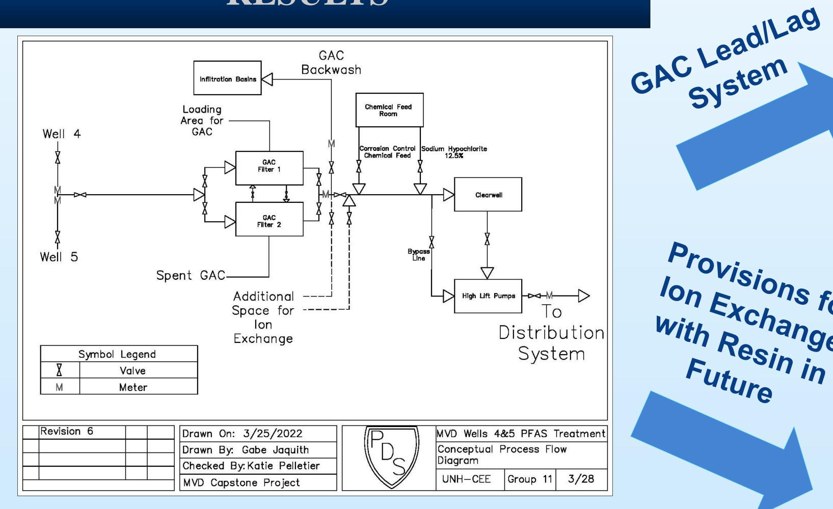
The flow diagram provides a basic overview of how the proposed treatment facility would operate. Through the diagram, we have illustrated the proposed treatment process and other key elements like backwashing and chemical feed.
