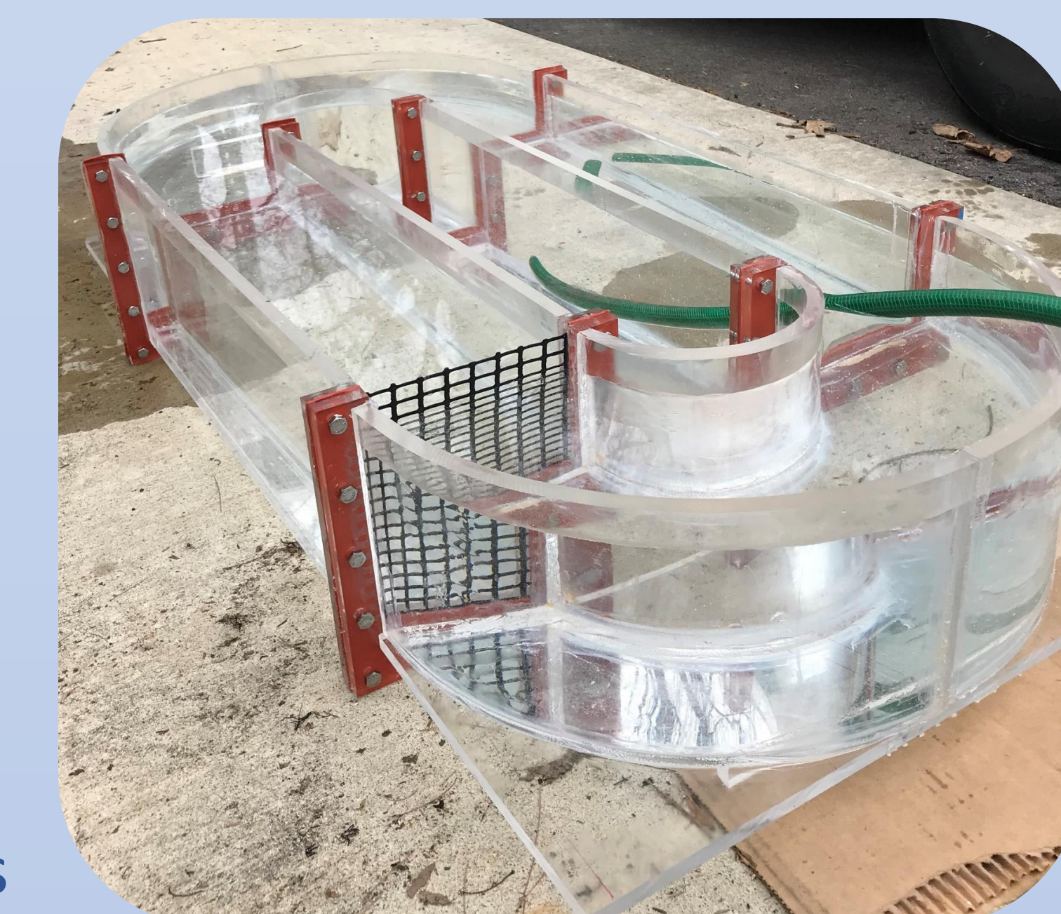
Flume Filled with Water for Testing
