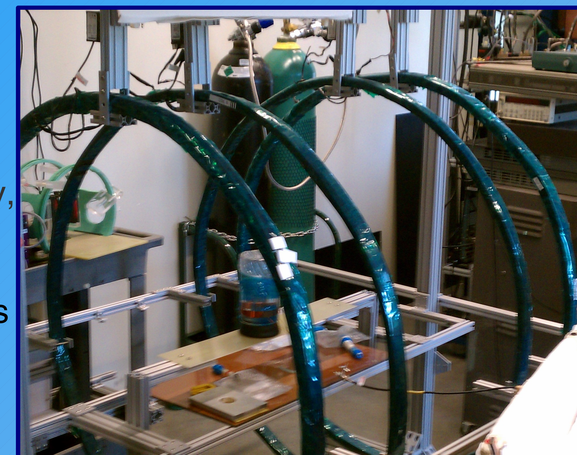
Figure 6: Experimental set-up of NMR water calibration. The probe sits in the middle of large copper coils which generate a uniform magnetic field required for Nuclear Magnetic Resonance. The magnetic field is controlled with the current created by a power supply.
