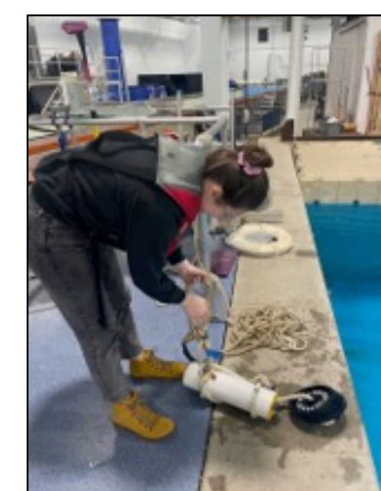
Figure 7: Left, students Anne Berg and Catey Selby manufacture electronics shelves for their instruments. Center, Anne prepares to test the waterproof seal on her instrument housing in the Chase Engineering Tank. Right, the same housing awaits testing under wave forcing in the Chase Wave Tank.
