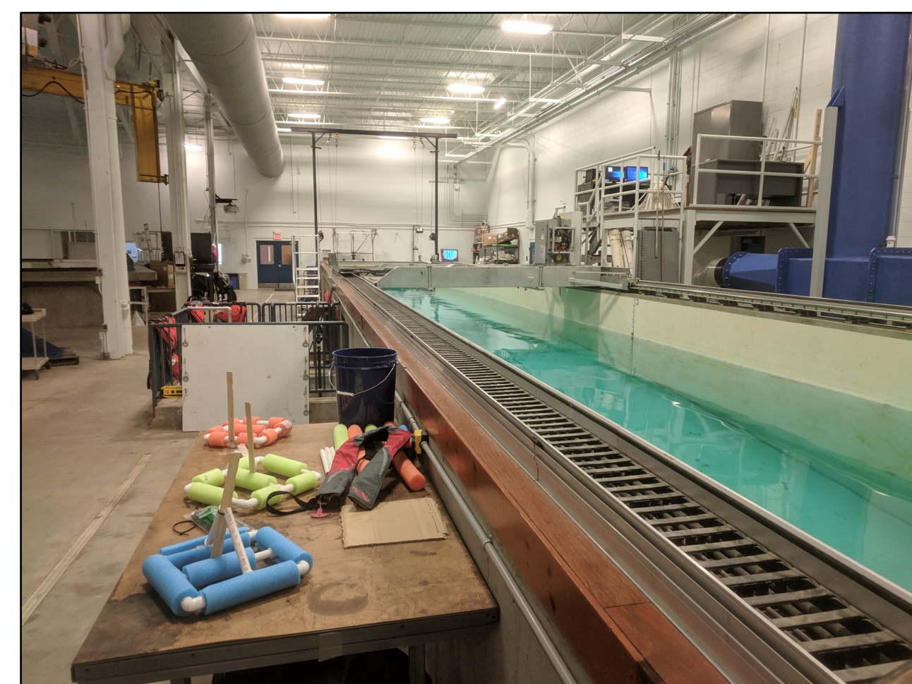
Figure 3: IMUs installed on simple floatation devices (bottom left) awaiting testing in the Chase Engineering Laboratory Wave Tank (right).
