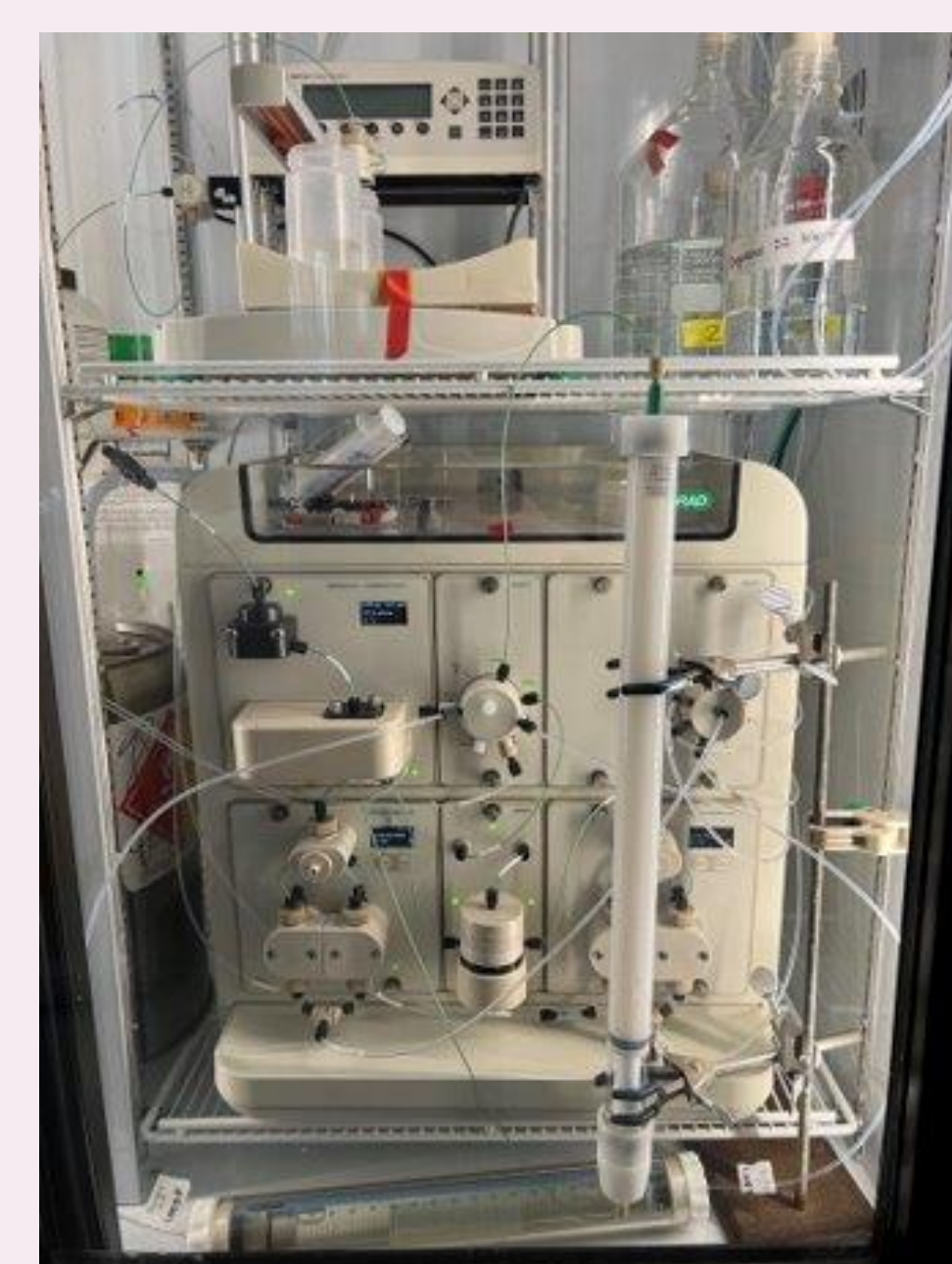
Figure 5 FPLC instrument with Anion Exchange Column
