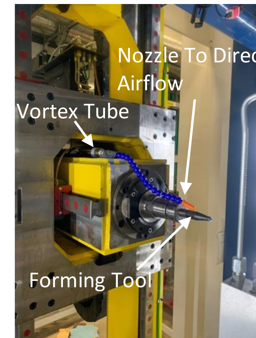
Machine spindle, vortex tube attached
