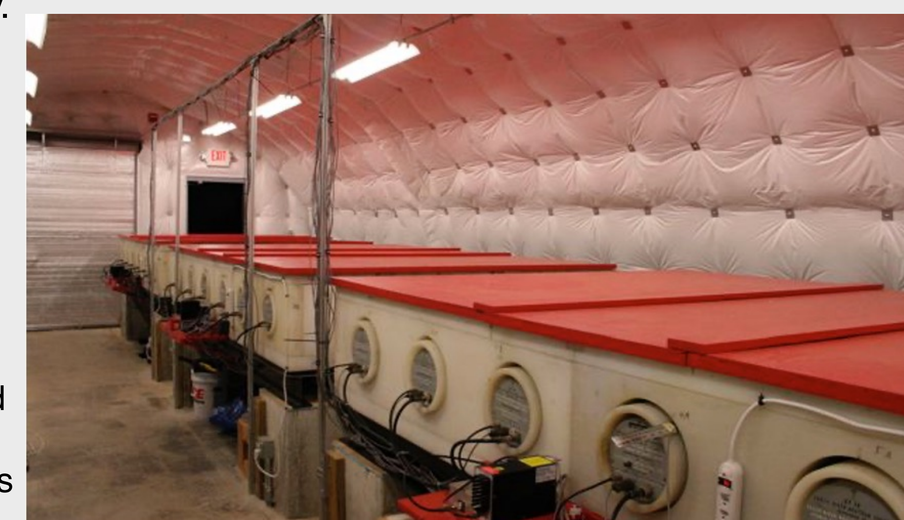
Figure 6: The 18 tubes of the Durham Neutron Monitor
