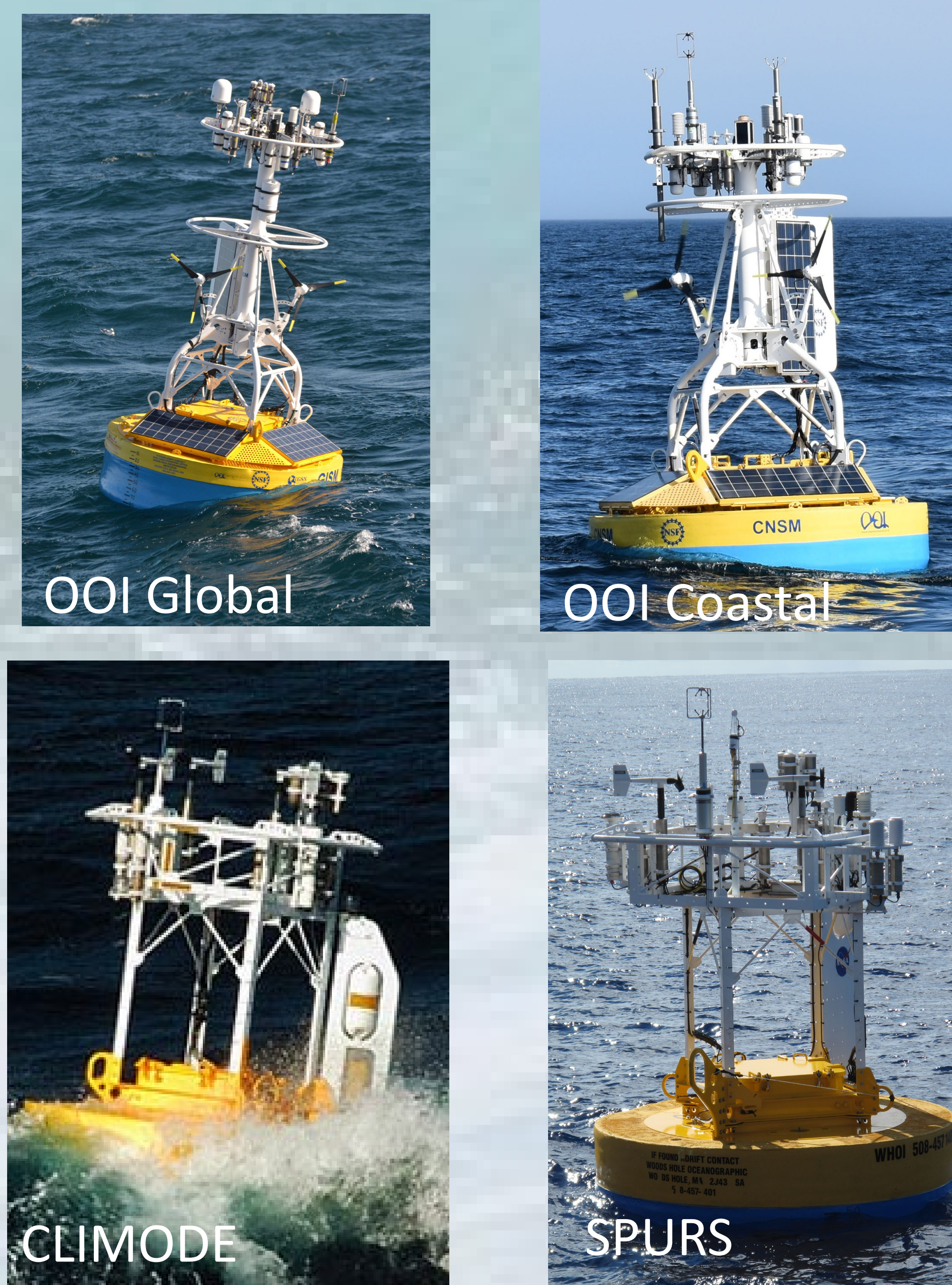
Figure 1 OOI Global and Coastal moorings and the CLIMODE and SPURS buoys. The OOI and CLIMODE buoys provide momentum and buoyancy fluxes. The SPURS buoy added an IRGA to directly measure the latent and sensible heat fluxes .
