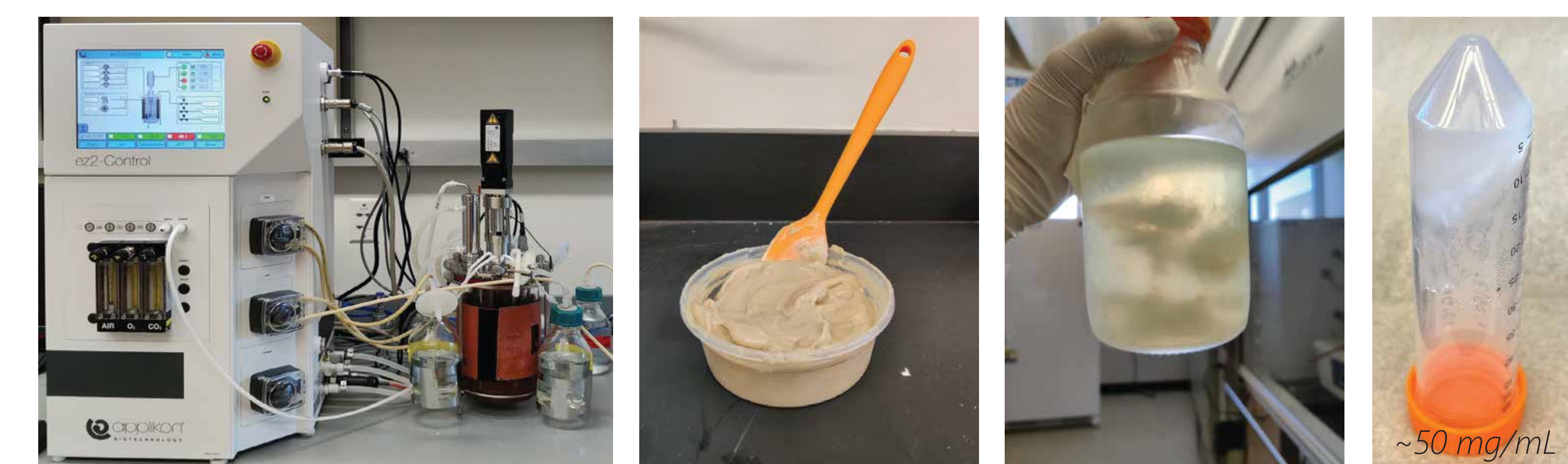
Applikon eZ 2 connect 3 and 7 L fermentation system allows for extensive optimization of growth profiles to maximize yield.
