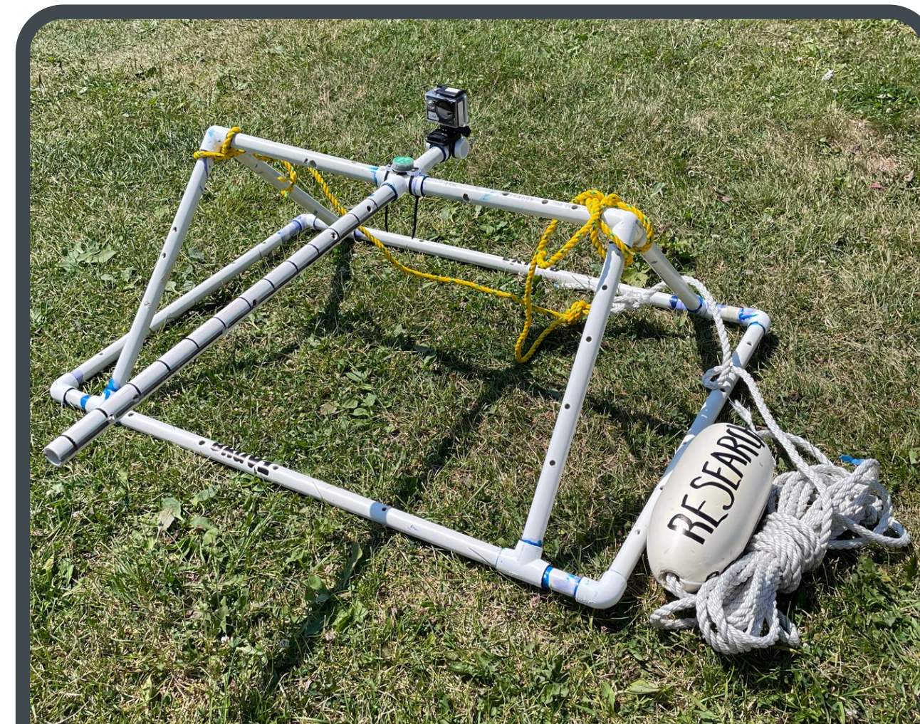
Figure 2: One of three identical RUVS used in this study. They are PVC structures that hold an AKASO EK7000 camera about a foot above the seafloor.
