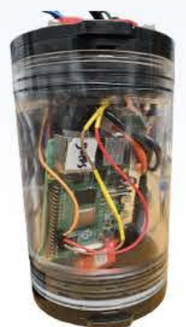
Fig 7. Waterproof enclosure and internal wiring
