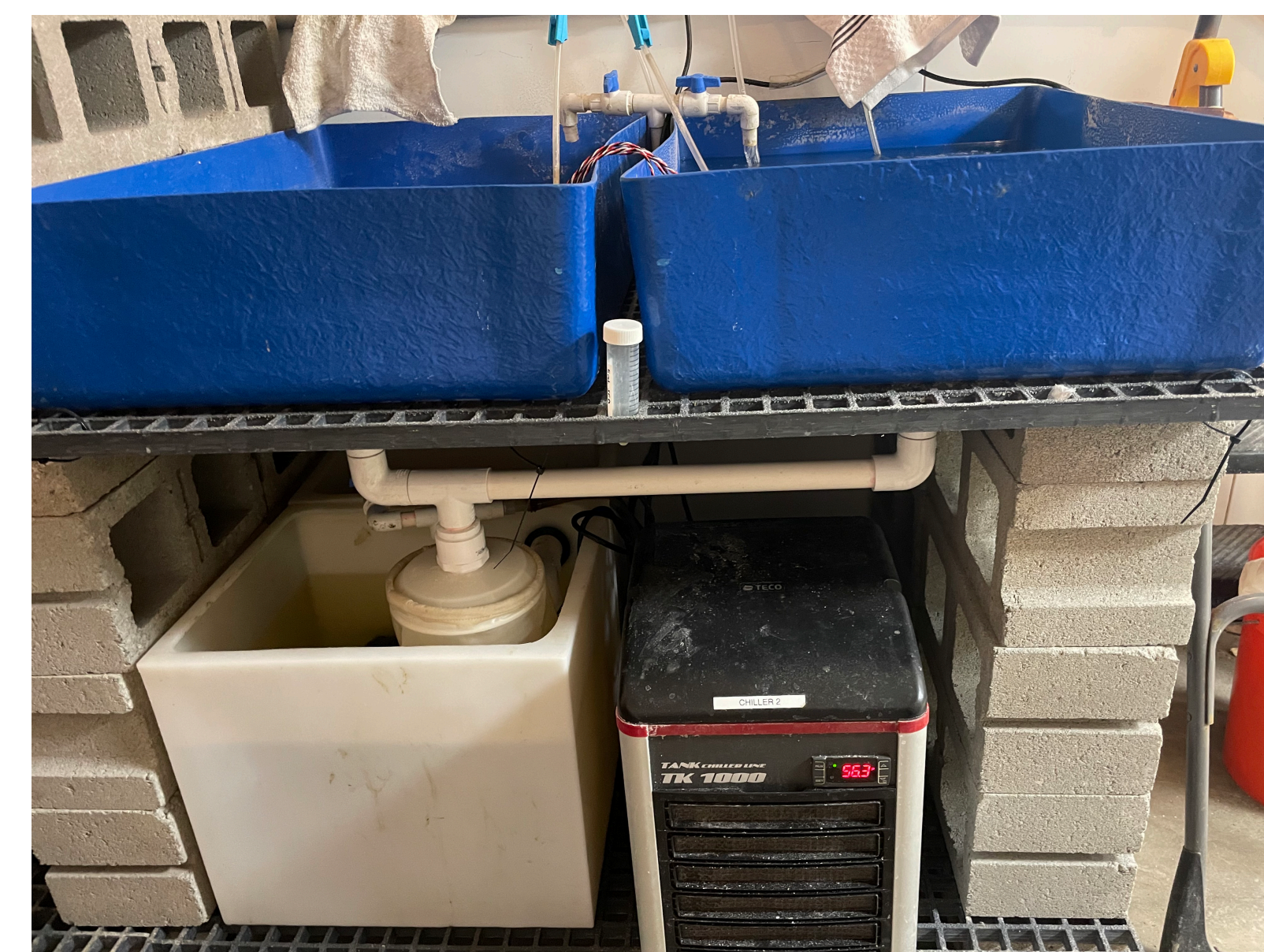
Figure 5. Kendall Hall experimental set up in flow through tank with bag filter, water pump, water chiller, and aerators
