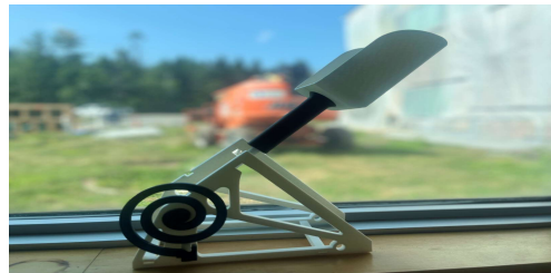
The prototype : (Left) The catapult/trebuchet launcher designed to toss bocce balls/beanbags. (Right) The stand the launcher attaches to for easy, stow away storage.
