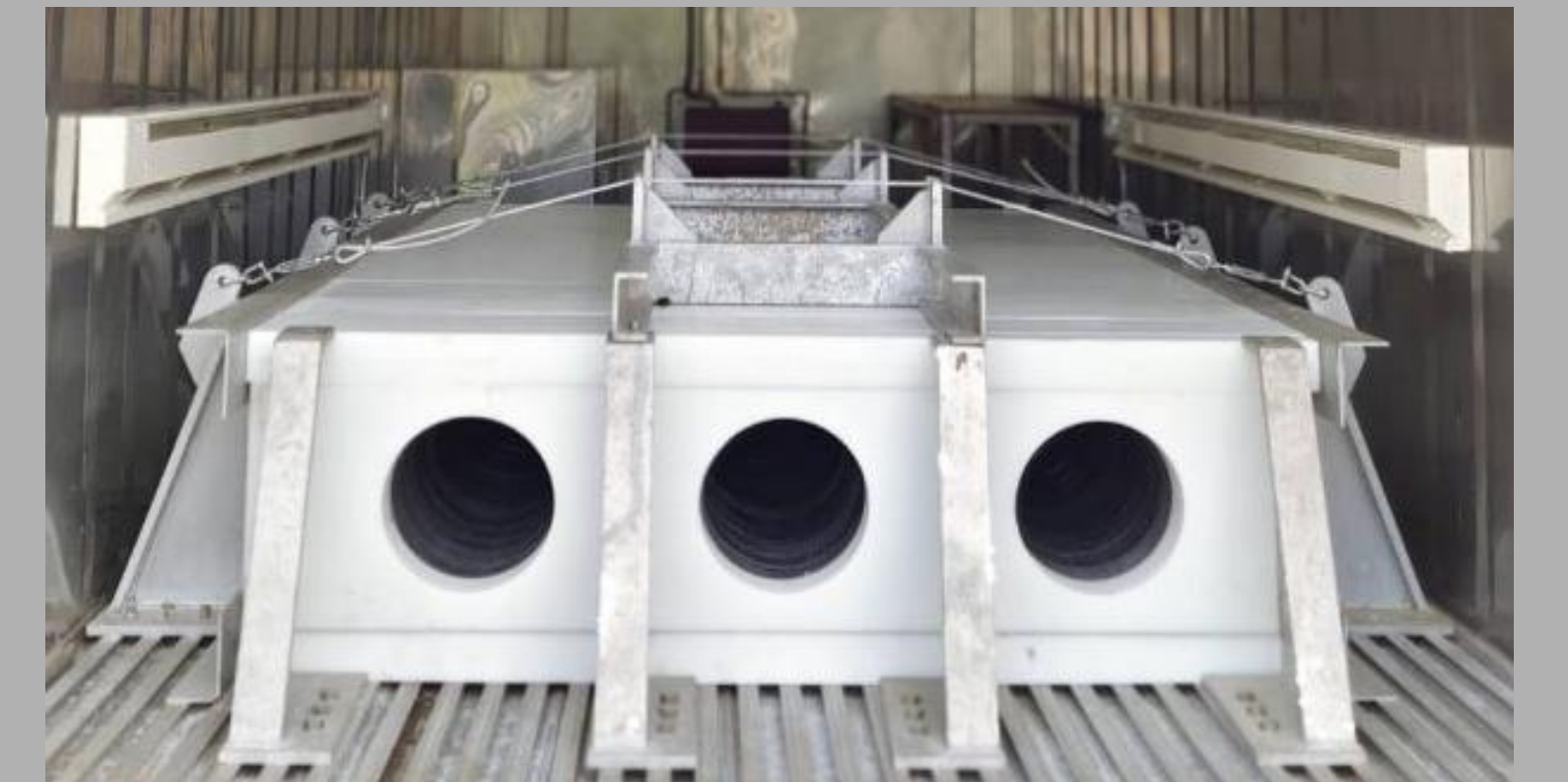
Figure 7. The Thimon monitor. The proportional counter tubes are not yet installed
