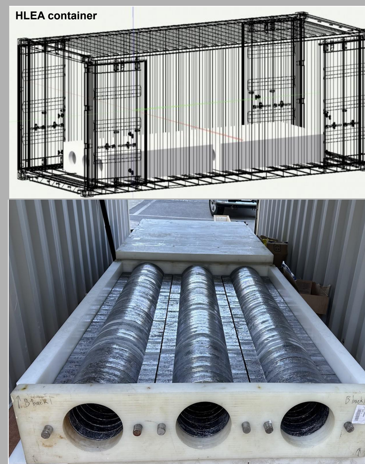
Figure 5. Top – a rendering of the shipping container and the positions of the housing for 2 banks of HLEA tubes. Bottom – a photograph of one bank of the HLEA monitor. The proportional counter tubes are still missing. The polyethylene reflector has been removed from the top to show the lead producer
